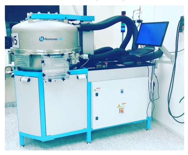
The unique clam-shell chamber design allows for easy access to the thermal test table making it easy for the test engineer to mount the test object and attached any diagnostic/control cabling that is required. The access ports can be customized to customer requirements.
